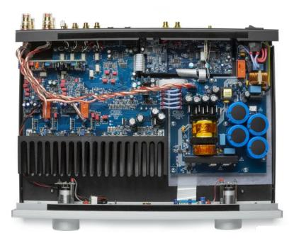
The power stage is based on six high current Mosfet Sanken STD03 transistors. To guarantee the advertised output power, CREEK has chosen a switching power supply. Thus, the designer is free from the conventional toroidal transformer (s) and filter capacitors.
