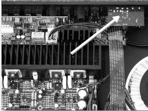
Line the plate up with the expansion slot in the rear panel. Using the screws previously removed, fix the RUBY module firmly onto the rear panel, using the Torx T7 screw driver, supplied in the pack.
