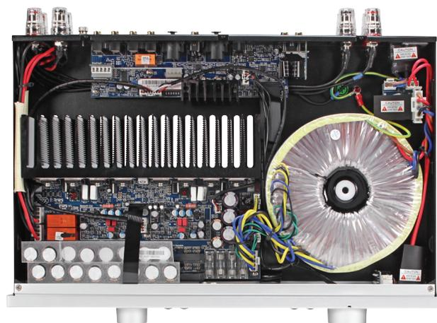
loudspeaker binding posts which can be selected individually or used in tandem – useful for those looking to bi-wire their ‘speakers.
